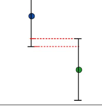
If the error bars for two average values don't overlap, a conclusion that they are different is justifiable. The **STANDARD DEVIATION** is a more sophisticated indicator of the precision of a set of *n* measurements:
