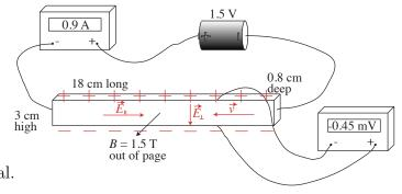
a. (2 pts) Draw an arrow indicating the direction of  $\vec{E}_{\parallel}$ , the electric field due to the battery and surface charges, which drives the the current in the bar. Label this arrow  $\vec{E}_{\parallel}$ .
