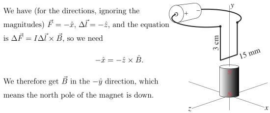
c. (7 pts) What is the magnitude of the magnetic field at the location of the 15 mm length of wire, due to the bar magnet? *Show all steps in your work.*
