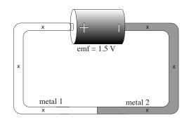
$5 \times 10^{-5}$  (m/s)/(N/C), and the electron mobility in metal 2 is  $2 \times 10^{-4}$  (m/s)/(N/C). The emf of the battery is 1.5 volts.
