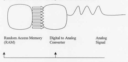
Control of rate at which DA converter pick and counters that picks address in RAM of digitized information.
