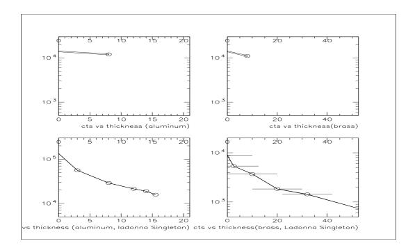
Figure 1: Collected X-rays from sodium source: no absorber, 8 mm aluminum, and 8 mm brass
