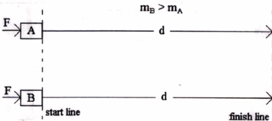
Suppose you allowed the sliders with different masses to travel the same distance  $d$  (the length of the track) while each is pulled by same tension force. PREDICT the following outcomes BEFORE doing the experiment based upon your knowledge of concepts related to energy and momentum.
