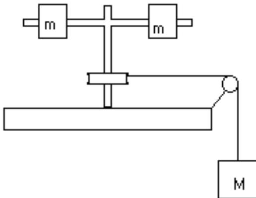
(1) Go to the apparatus that consists of two adjustable masses  $m$  on a light horizontal rod which can rotate about a central vertical axis. The distance of masses  $m$  from the axis of rotation can be adjusted. The central rod is attached by a string to a mass  $M$  which provides a tension in the string. This tension force in turn causes a torque about the central axis which results in an angular acceleration of masses  $m$ .
