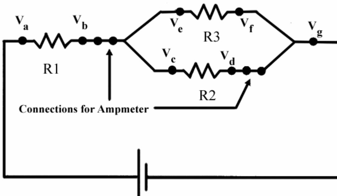
The DC voltage supply should be set to 10V (check the dial to be sure). Since the resistors are all at least 1kΩ, the currents are a few milliamps (mA). The purpose of this exercise is to find the values of the resistors, the voltages at various points, and the currents in each part of the circuit.
