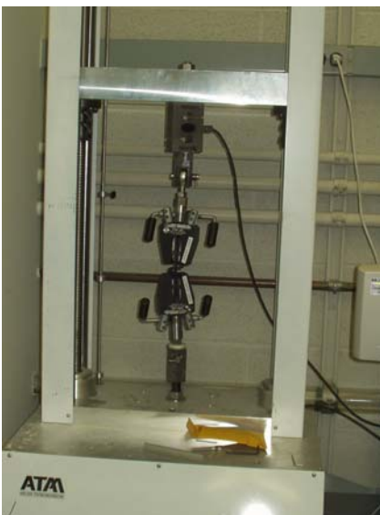
Figure 5: Our machine used for tension test.
