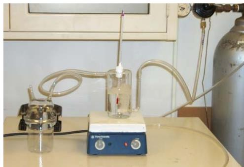
Figure 4: Water saturated nitrogen at 60°C
