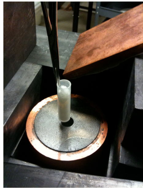
Pb-210 screening in PZT Pb oxide (low-bckg HPGe "well" detector)
