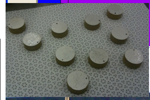
Pb-210 screening in PZT Pb oxide (low-bckg HPGe "well" detector)
